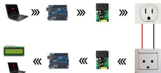
Fig:5.2.1 Block diagram of PLC system
